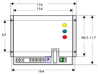
height=37mm, d(fixing drills)=5mm
